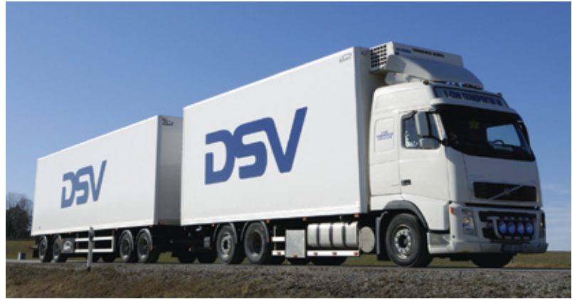
One of the new heavy goods vehicles of DSV measuring 25.25 metres. It can carry three 20-foot containers, thereby contributing to less road traffic and reduced CO 2 emissions.
