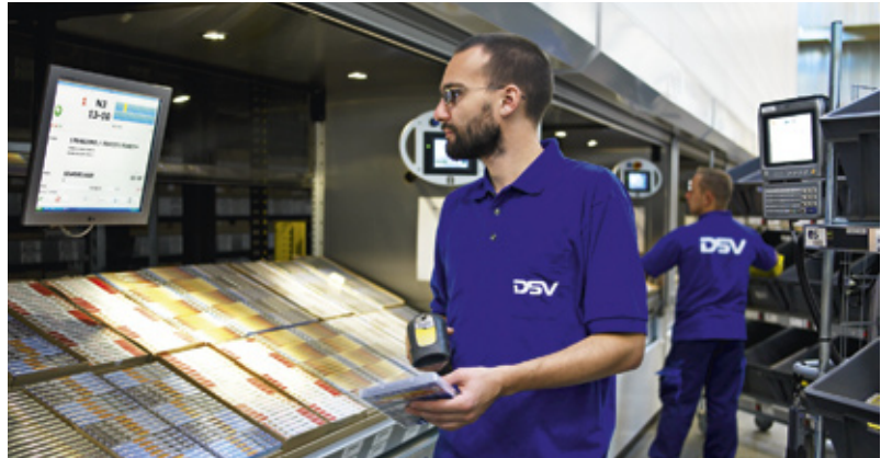
The operation of a LogiMat vertical lift. The LogiMat is used to pick the individual items for an order, e.g. auto spare parts. The system verifies that the weight of the individual item picked is identical with the weight data stored.
